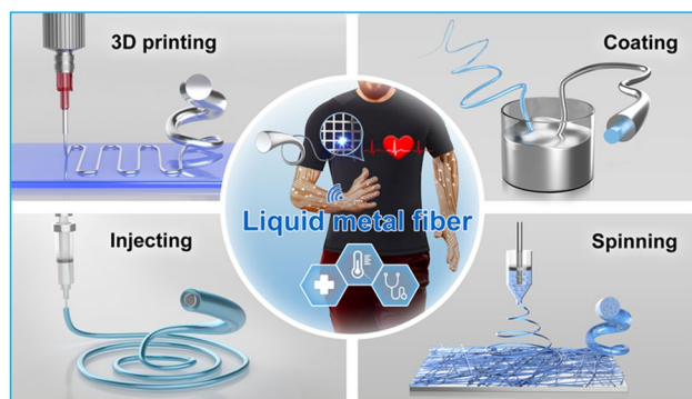
Fig. 1 Schematic illustration of a liquid metal fiber and its fabrication technologies
