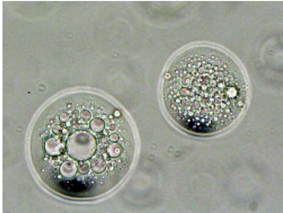
Fig. 17 Presence of multiple emulsions (water-in-oil in water) after the occurrence of inversion.
