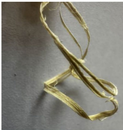
(c) Bamboo fibers treated with calcium hydroxide solution
