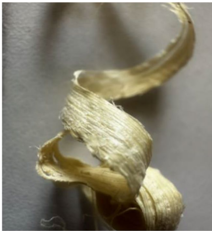
(a) Bamboo fibers treated with water
