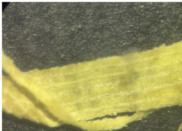
(d) Microstructure of bamboo fibers treated with calcium hydroxide solution
