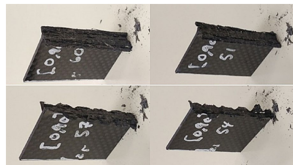
Fig. 18 Isometric views of Dyn crush tests for Hat-Shape coupons with [0/90] 2s layup; (top): coupons with chamfer45 and steeple trigger, (bottom): coupons with corrugated and saw teeth trigger
