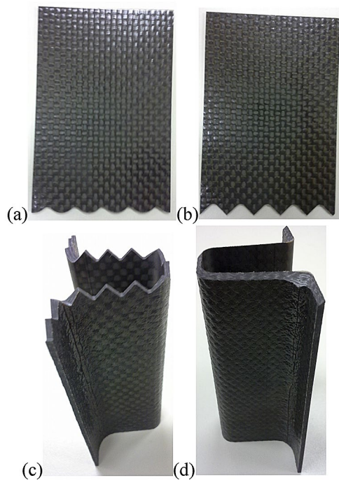
Fig. 9 a Flat-plate coupons with corrugated trigger, b flat-plate coupon with saw teeth trigger, c Hat-Shape coupon with saw teeth trigger. d Hat-Shape coupon with chamfer45° trigger
