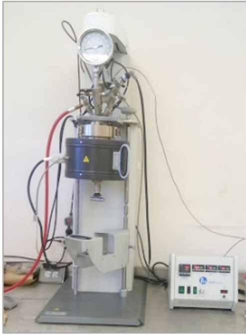
Fig. 2 Parr titanium reactor with a 1 L capacity (Mod. 4523)
