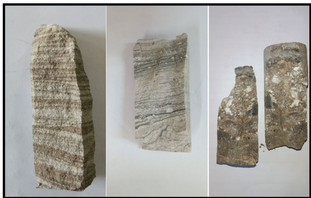
Fig. 1 Images showing heterogeneous structure as well as impurities in the specimens after UCS test
