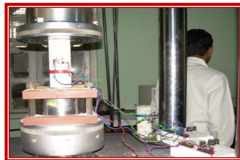
Fig. 6 Laboratory testing for determining Young’s modulus
