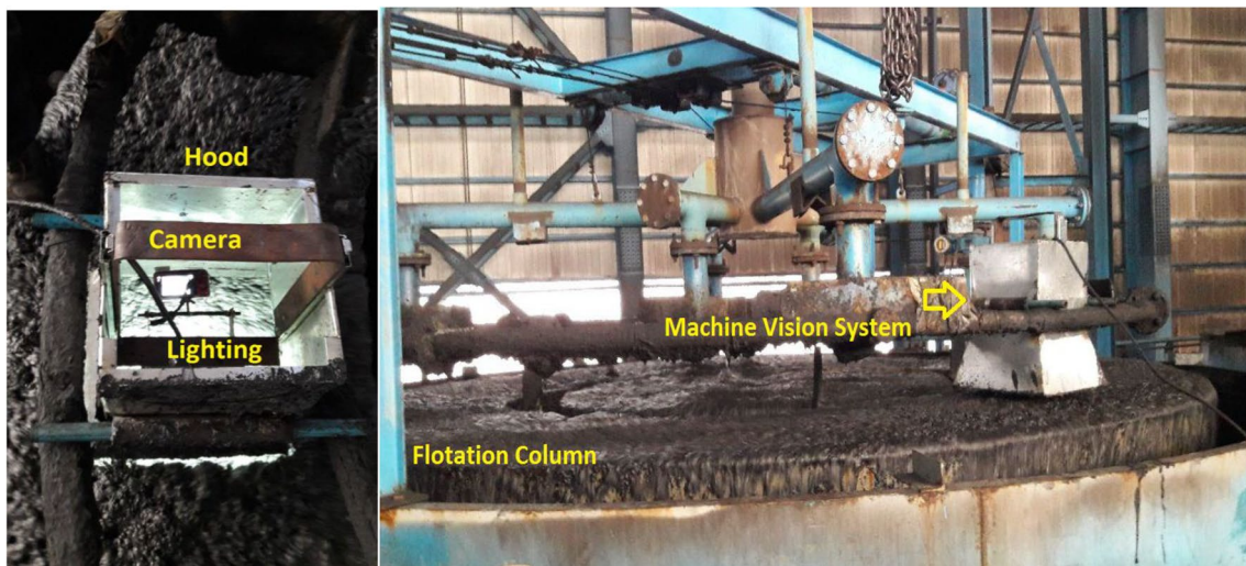
Fig. 9 Coal flotation column and machine vision system [18]
