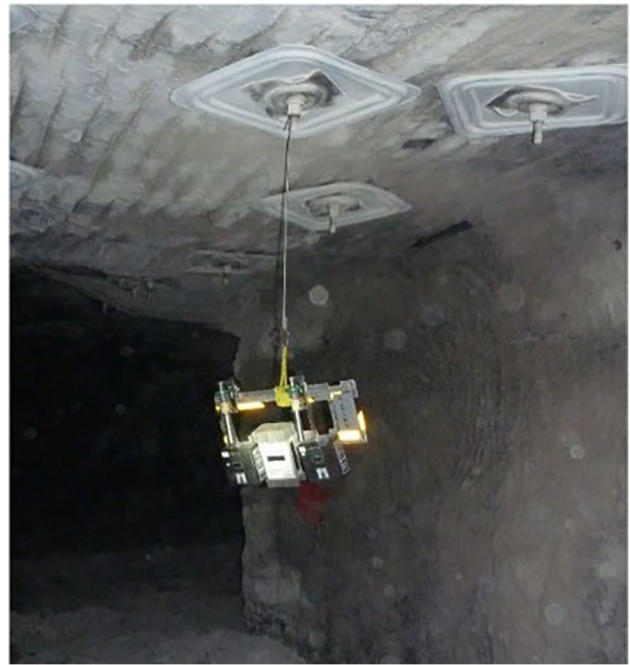
Fig. 6 A typical gravimetric sampling package consisting of a pDR-1000 and two gravimetric samplers. This package is typically hung from a roof bolt or mounted on mining equipment
