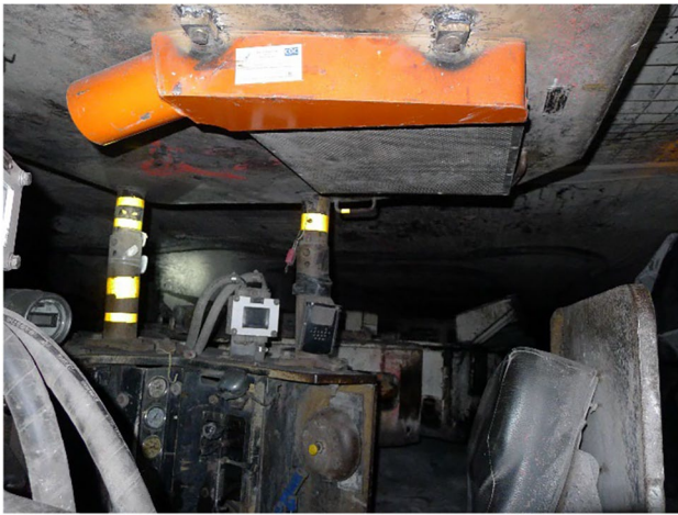
Fig. 2 Air curtain plenum welded to underside of ramcar canopy located above the operator's seat
