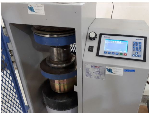
Fig. 3 The piston-die cell under pressure
