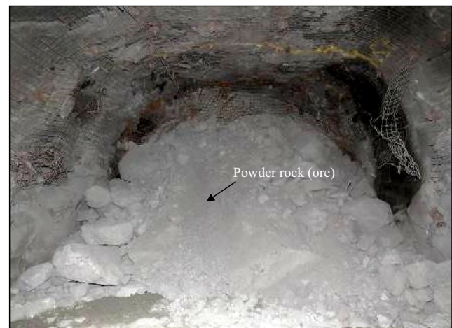
Fig. 2 The powder rock (ore) enters the drawpoint
