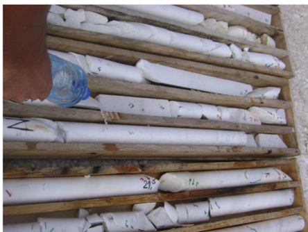
Fig. 5 Drill cores of HQ diameter in the wooden boxes. All the cracks were identified and colored according to the set they belong to. Some cores have been sawed in the processing plant along their axial plane for inspection of the color and other defects. Each of the three series of cores inside each box has as length of 2 m to facilitate core measurements
