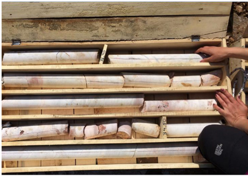
Fig. 6 HQ (63.5 mm) marble cores with the top line along the core-axis marked on them
