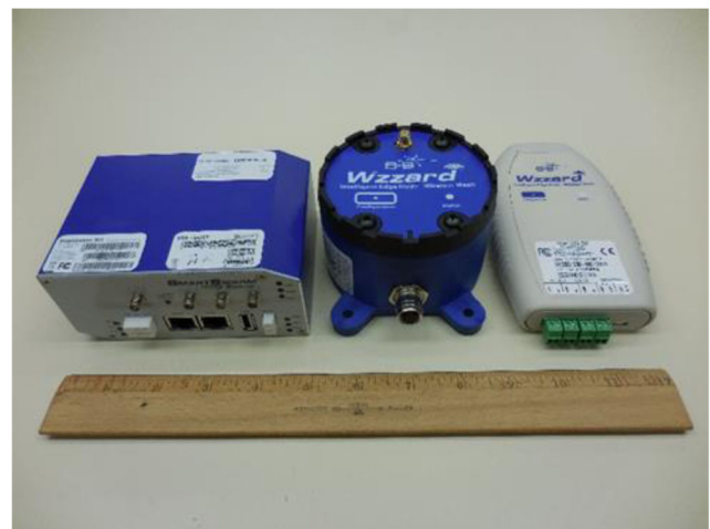
Fig. 3 A SmartSwarm cellular gateway (left), industrial-grade Wzzard node (middle), and commercial-grade Wzzard node (right)
