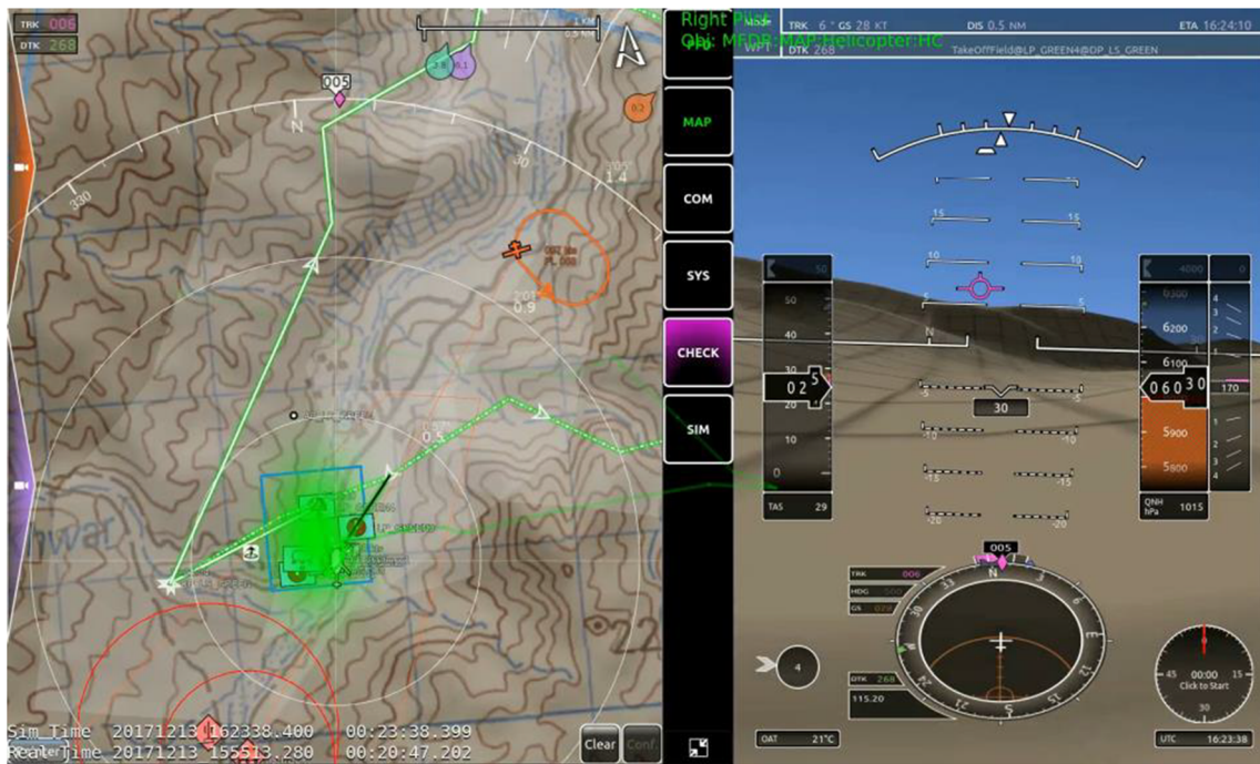
Fig. 11 Multifunction display of the right pilot with the tactical map on the left and the primary flight display on the right. The pilot’s green gaze point (including the local gaze measurement accuracy as a Gaussian distribution) is located at the helicopter on the tactical map.
