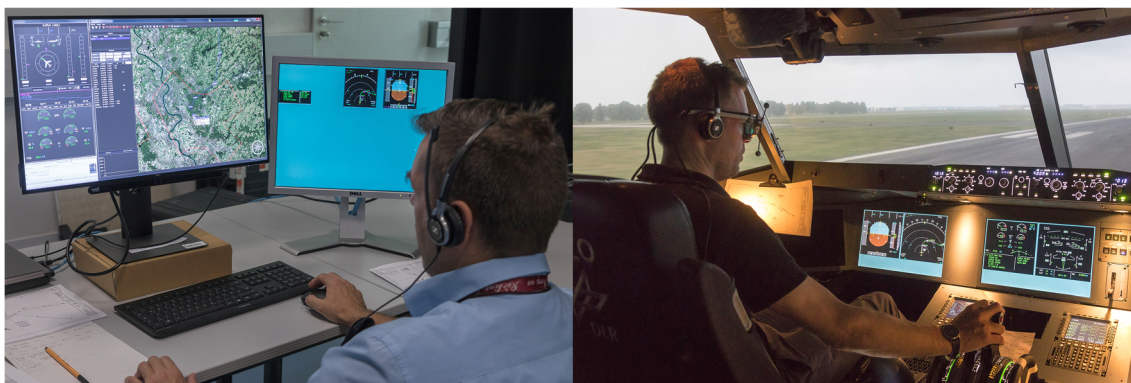
Fig. 1 The two experimental conditions: (left) the remote-copilot at the ground station and (right) the Captain on the multi-crew flight deck (only one pilot on the flight deck in RCO)
