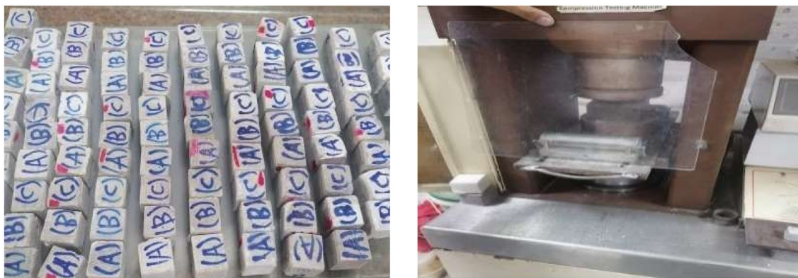
Fig. 3 Cubes in aggressive media, extracted and broken in a compressive strength machine
