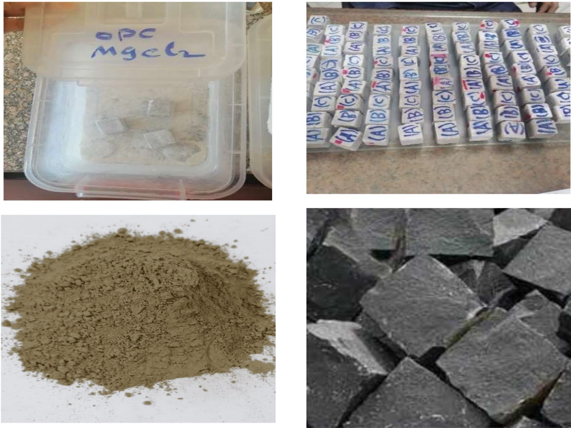
Fig. 1 Cubes immersed in 5% MgCl_2 and BP as raw material
