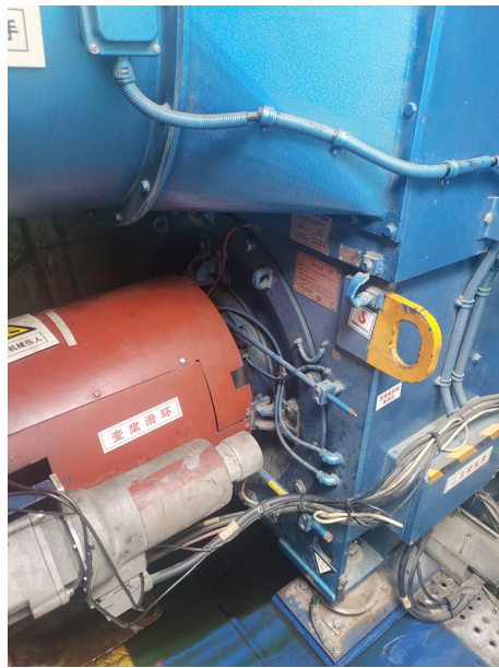
Fig. 5 Data acquisition of wind turbine bearing
