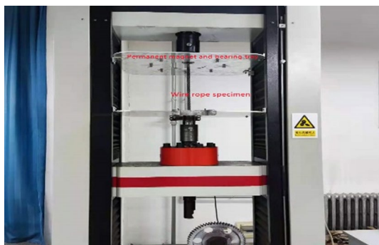
Fig. 13 Force-magnetic coupling test equipment
