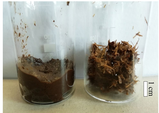
Fig. 3 Wheat straw slurry for SFS (left) and LFS (right) after 12 h hydrolysis time at 20% DM solid loading
