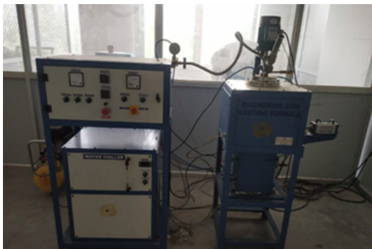
Fig.3 Stir casting machine for fabrication of composite
