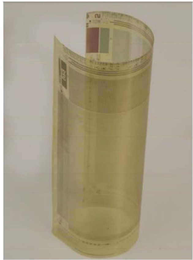
Fig. 6 50 \times 50 mm a-Si TFT array on 3 \mu\text{m} thick freestanding polyimide layer made by the EPLaR process [107]
