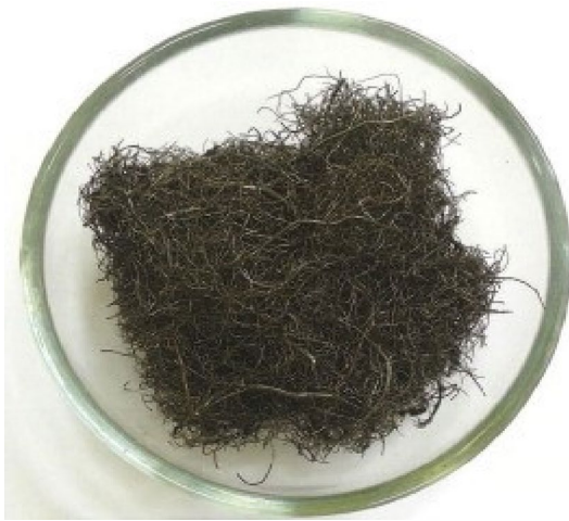
Fig. 4 Extracted steel fibers
