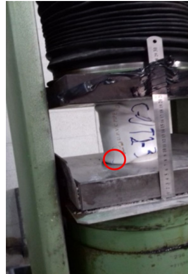
Fig. 10 Ductile failure of C-OJT
