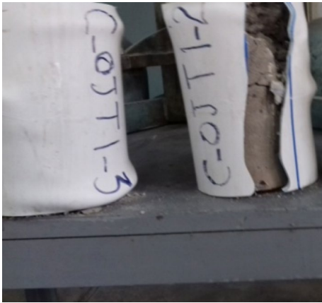
Fig. 11 Brittle failure of C-OJT
