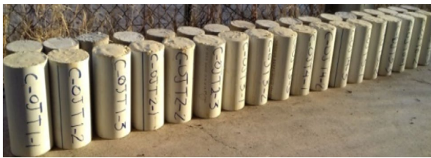
Fig. 3 Capping of top of C-OJT specimens
