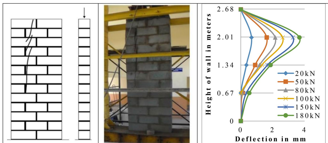
Fig. 7 Views of failure patterns and distribution of lateral deflection along the height at various stages of loading of wall no. 3 (HCB-200-A3)
