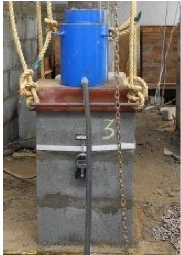
Fig. 3 Typical test setup for testing concrete block prism
