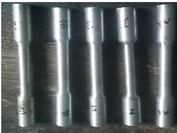
Fig. 1 The tensile test sample geometry
