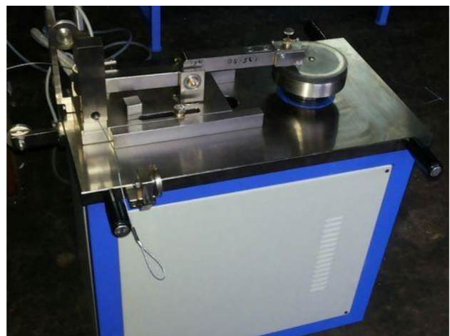
Fig. 2 Pin-on-disc wear tester
