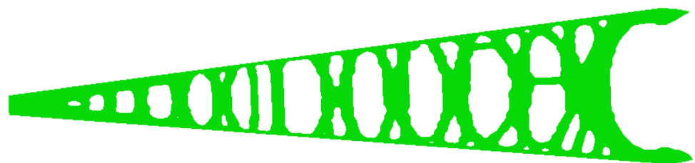
Fig. 15 The optimum layout of the stiffened structure
