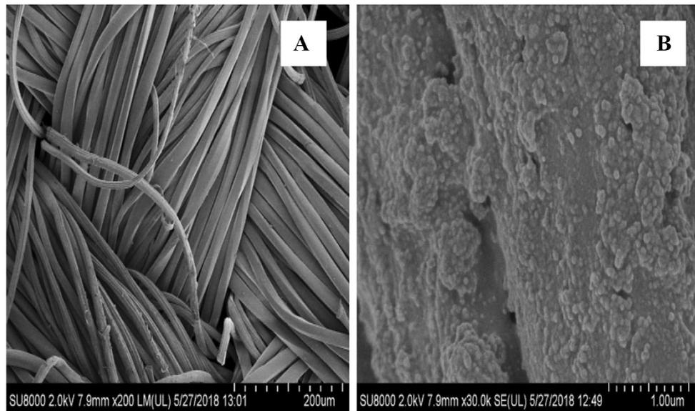
**Fig. 5** FESEM image of the textile fabric surface, with **a** 100% polyester before binded AgNPs and **b** 100% polyester after binded AgNPs at 30 k magnification
