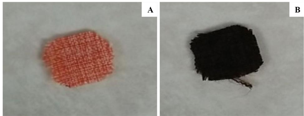
**Fig. 2** Transformation of colour on the surface of textile fabric, with **a** 100% polyester before binded AgNPs and **b** 100% polyester after binded AgNPs
