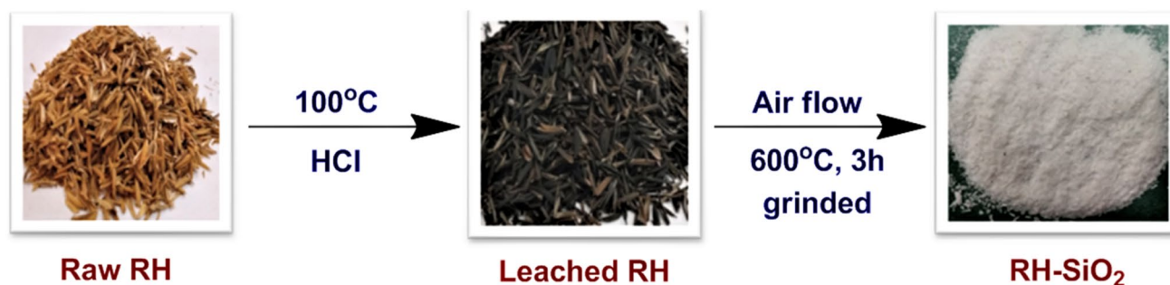
Scheme 1 Preparation of rice husk derived silica (RH-SiO 2 )
