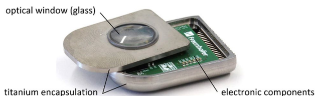
Fig. 1 Implantable medical implant with functional glass windows
