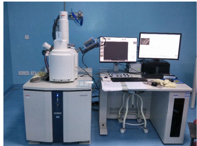
Fig. 4 Setup for SEM-EDS measurements
