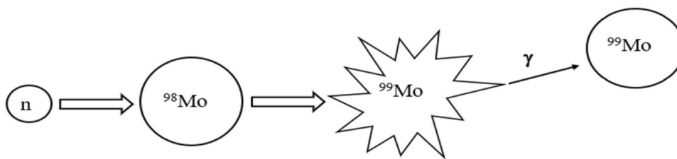
Fig. 3 The neutron activation of ^{98}\text{Mo} to generate ^{99}\text{Mo} [19]
