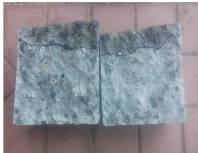
Fig. 5 Split concrete cubes after permeability test
