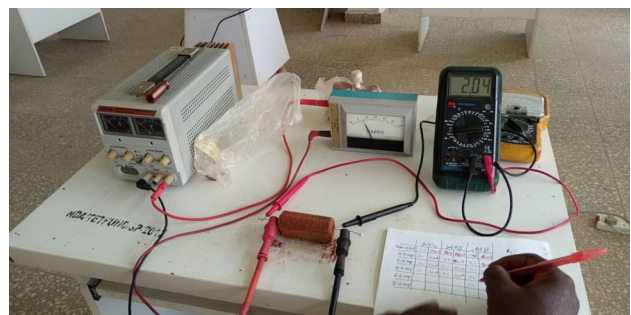
Fig. 1 Soil resistivity testing system utilized in this research
