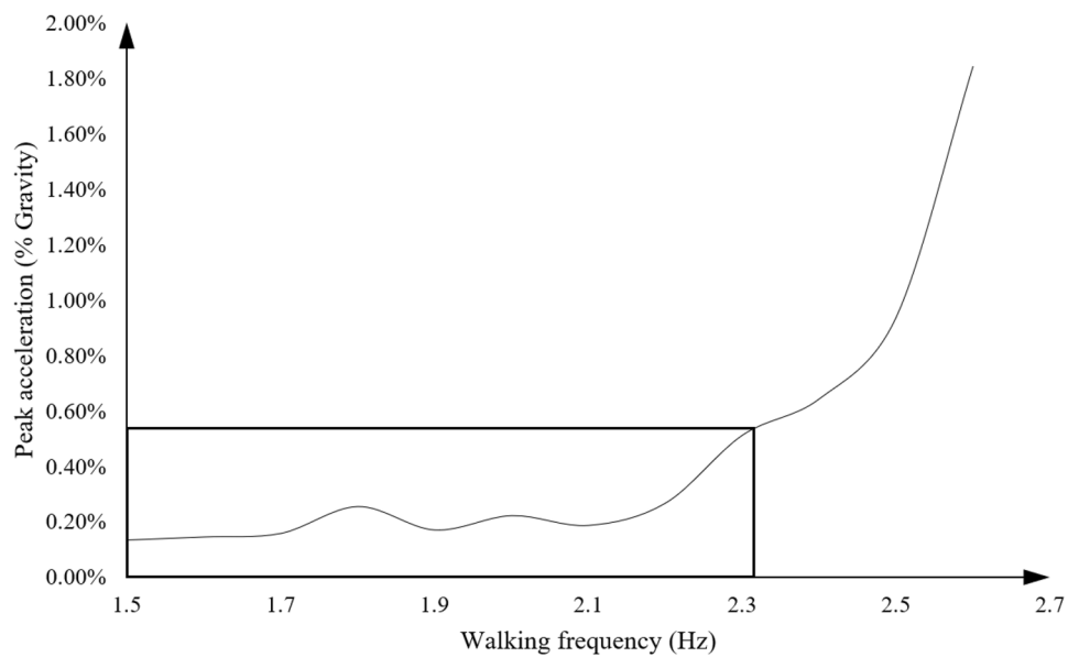
Fig. 10 Peak acceleration verse walking frequency (LM-2-3) for the slab with a thickness of 150 mm
