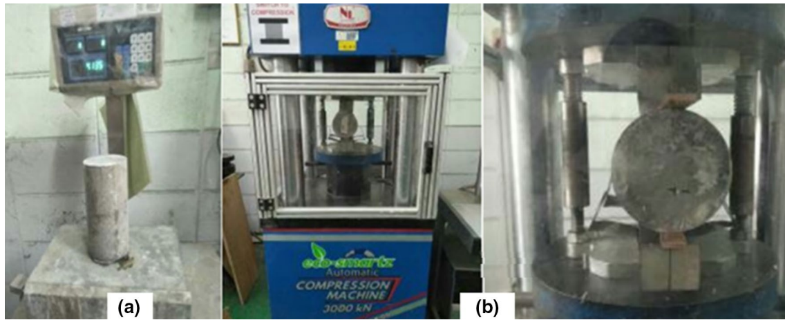
Fig. 3 a weighing of the specimen prior to testing and b Splitting tensile test
