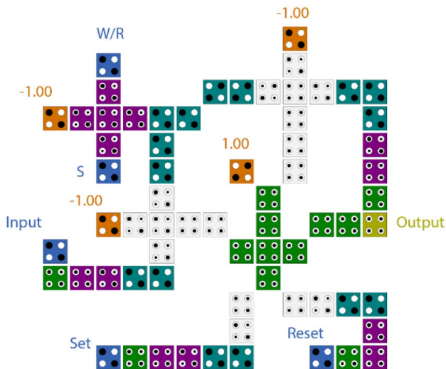
Fig. 12 The proposed structure of QCA-RAM cell
