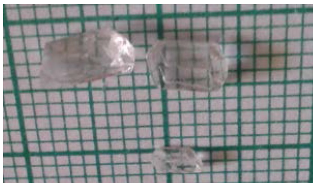
Fig. 1 Photograph of the grown LLZS crystal
