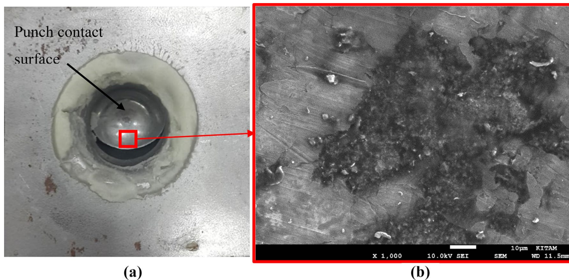
Fig. 5 a A specimen with 7.5 wt% SiO 2 nanolubricant after the Erichsen test; b a randomly selected punch-sheet metal contact surface
