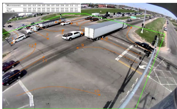
Fig. 3 An example scenario from the AI City Challenge vehicle counting dataset designed for multi-class, multi-movement vehicle counting
