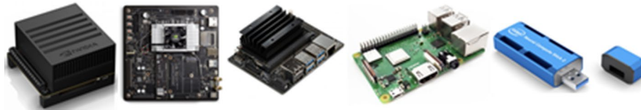
Fig. 4 Hardware (left to right): NVIDIA Jetson Xavier (Jetson AGX Xavier Developer Kit 2020), NVIDIA Jetson TX2 (Jetson TX2 - Elinux.Org 2020), NVIDIA Jetson Nano (Jetson Nano Developer Kit
