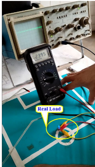
Fig. 10 Real load measurement (single load) connected to the voltage doubler circuit by Avometer and Oscilloscope
