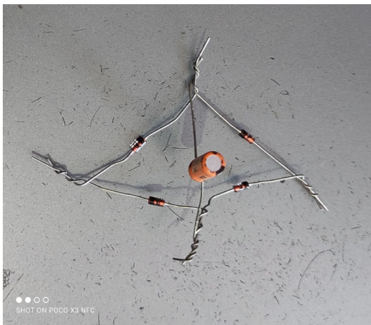
Fig. 6 Prototype of a bridge rectifier circuit + filter
