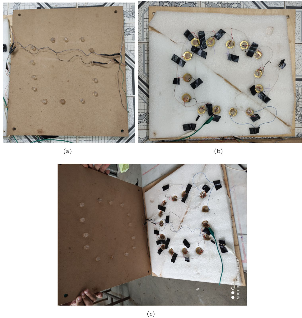
Fig. 5 Experimental setup of the proposed footsteps energy harvesting system (a) Wood plate No. 1, (b) Mounted piezo-electric elements on the foam and wood substrate plates, and (c) 3 plates
