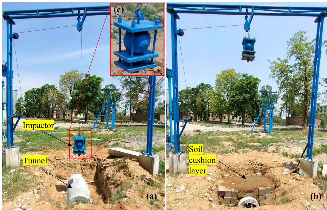
Fig. 2 Experimental setup of a bare tunnel b tunnel with soil cushion layer and c drop weight impactor
