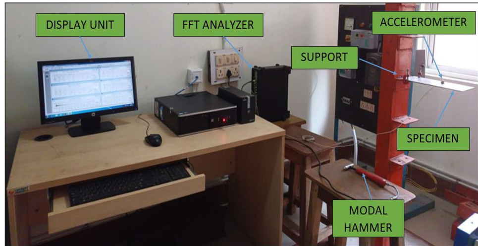
Fig. 2 Photograph of the experimental set-up for modal testing of the sandwich plate under a clamped-free boundary condition
