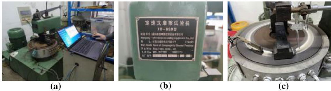
Fig. 13 XD-MSM constant speed friction tester
