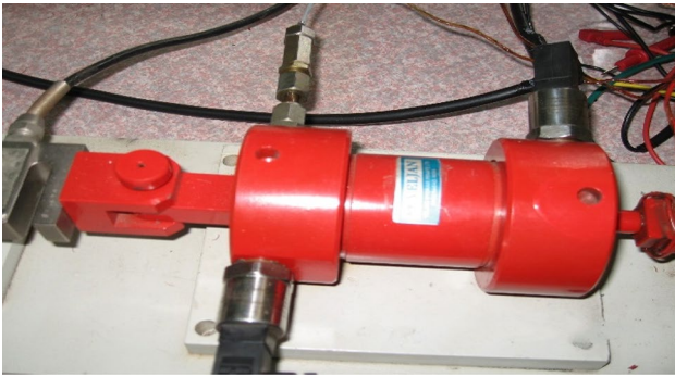
Fig. 3 Small capacity MR damper filled with nano magnetorheological fluid
