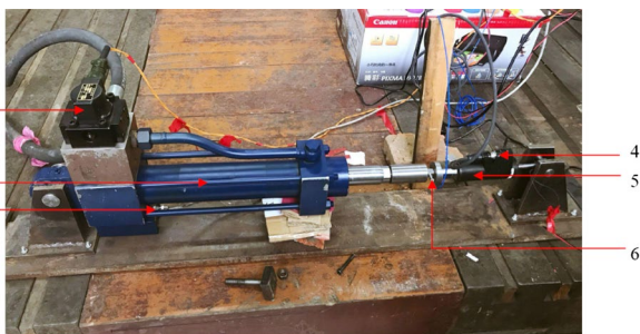
1. Electromagnetic hydraulic valve 2. Servo cylinder 3. Motion detector 4. Speed sensor 5. Magnetorheological damper 6. Force sensor
