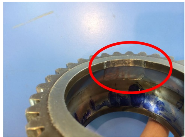
Fig. 4 Slot across the bearing outer race
