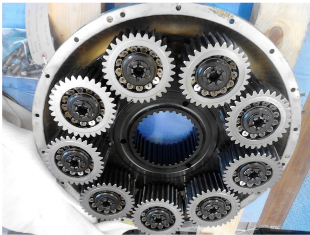
Fig. 3 Second-stage epicyclic gears
