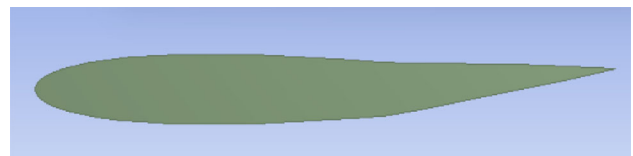
Fig. 32 NACA 0012 trailing edge morphing length at 60% of chord for -5^\circ bending angle
