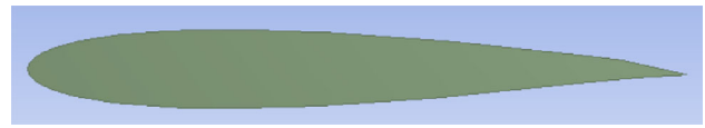
Fig. 29 NACA 0012 trailing edge morphing length at 90% of chord for 5^\circ bending angle
