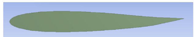
Fig. 31 NACA 0012 trailing edge morphing length at 80% of chord for -5^\circ bending angle
