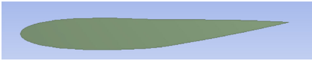
Fig. 33 NACA 0012 trailing edge morphing length at 50% of chord for -5^\circ bending angle
