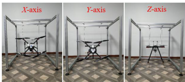
Fig. 7 The test platform designed to assess rotational inertia
