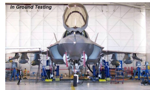
a) BF-3 during Structural Coupling Test
